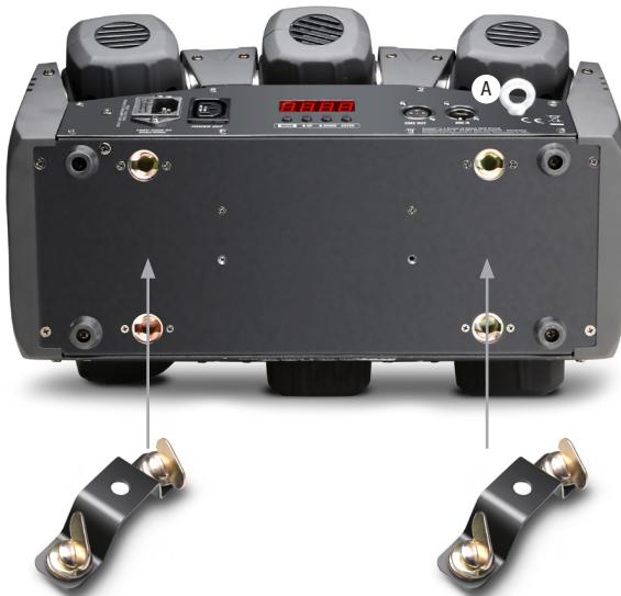
**EN** Thanks to the integrated rubber feet, the spotlight can be placed in a suitable location on the stage floor etc. Mounting on a truss is performed with the help of the supplied omega mounting bracket (truss clamp not included). Overhead installation should only be carried out by trained personnel. The spot must be secured with an appropriate safety cable to the safety eyelet (A) to prevent falling.
