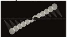
Pull Middle - The first and last selected fixture remain at the current value, the midpoint is affected most. This is useful for colour mixing, tilt and dimmer.
