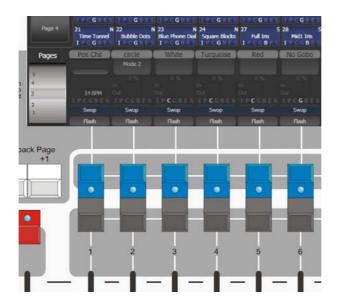
A Static Playbacks workspace is available to show the contents of the macro/executor buttons and (on the Tiger Touch) the 10 static playback faders.
