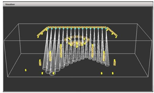
The console runs Avolites Visualiser internally. This allows you to view the output of the console if you can't use the real lights, enabling you to make changes to your show at home or in your hotel. It can also be used in Blind mode for programming during a show.
