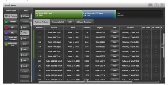
**Fixture type:** lists the different types of fixture in your show. Each fixture has a unique colour code. Click on these buttons to select all fixtures of the type.
