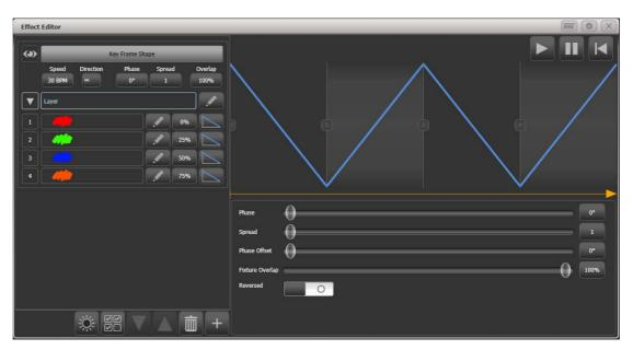
The controls at the top of the left hand pane are the global shape properties which affect the whole shape, controlling speed, direction, phase/spread and fixture overlap. The eye icon in the top left corner "collapses" the shape preview in the effect editor window, this allows you to expand only the shape you want to work on if you have created multiple shapes.
