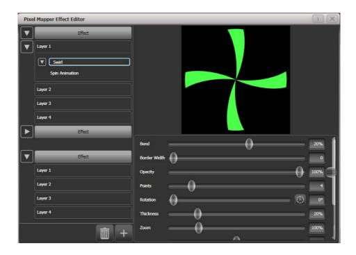
To see how the effect will look on the fixtures, open the Pixel Mapper preview window by pressing View, [Open Workspace Window], [Pixel Mapper Preview]. A real life view of each effect running is shown in a button at the bottom of the screen, you can select each of these by pressing the button.
