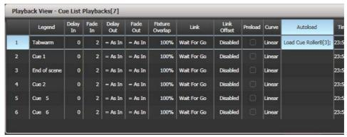
The Autoloaded playback will be fired when the cue starts, and killed when the cue list moves on to the next cue, unless you have also loaded the playback into the next cue.
