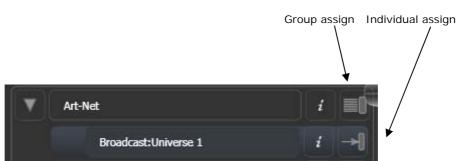
To assign a node to a line, click on the arrow on the node (the node will be highlighted), then click the line you want to assign to it.
