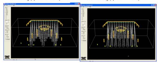
The display above the left hand wheel shows the phase in degrees. For example, 180 degrees repeats every 2 fixtures, 90 degrees repeats every 4 fixtures, 60 degrees repeats every 6 fixtures, and so on.
