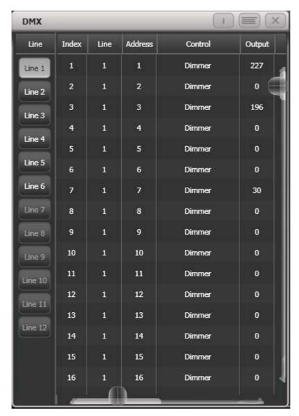
The buttons on the left let you select the different output lines from the console. Scrolling the window to the right shows more information about each DMX channel.
