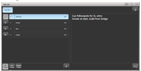
A set list is made up of tracks. When a track is added it automatically links to the current page. Pressing the play button next to the track will automatically select the correct playback page (except on Pearl Expert, because the rollers cannot be moved automatically).
