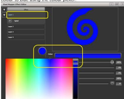
5> Select the Layer to show the layer controls and change the colour to blue using the colour picker.
