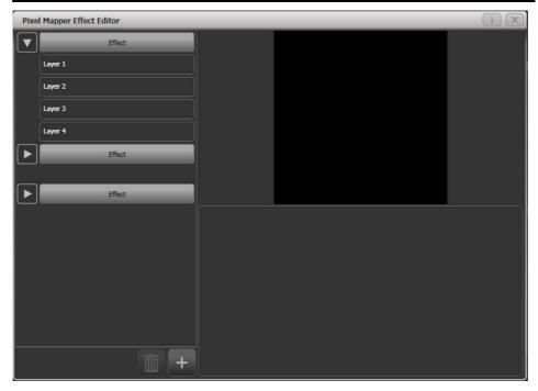
Click on the + button at the bottom to add an effect, and choose a graphic element. The graphic buttons as shown below provide the following effects:
