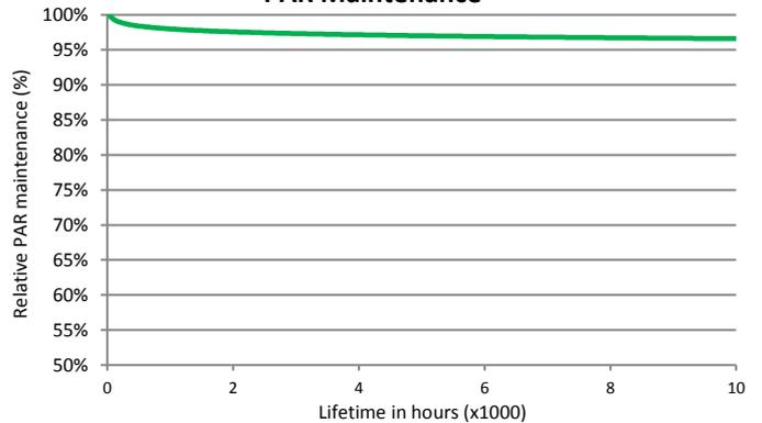
— BLV HORTURION HPS 1000W DE EL (the trend line is based on tests under defined and stable laboratory conditions. Measurements are performed on naked lamps in a Ulbricht sphere with a Licor LI 190)
